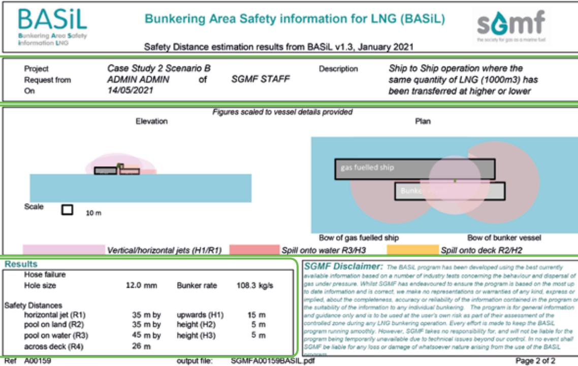
**Part E:** Includes a simplified graphical representation of the safety zone for the given parameters and bunkering scenario.
